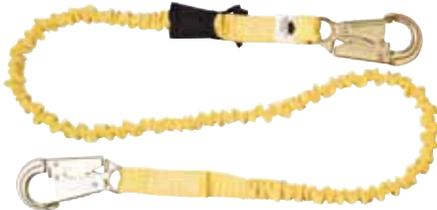
These lanyards feature a tubular, energy absorbing inner core that uses the entire length of the lanyard to absorb the energy of a fall and reduce the arresting forces on a user.
